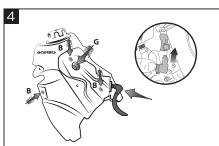
Place the Acerbis fuel tank (A) on the bike. Insert the tank and seat screws (G/B) as indicated in the diagram. Reconnect the fuel pump power cable and the fuel connector.
