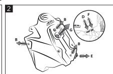
Remove seat screw (B) and the screws on the side. Remove the tank screw (G), then empty any remaining fuel from the tank. Remove the (D/E/F) fasteners and remove the fuel pump. Togliere le viti (B) della sella, e degli
