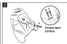
On the fuel tank Acerbis (A), reconnect the fuel pump (E) with the original screws/ hardware.
